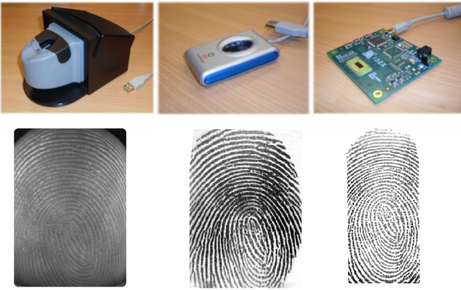
Fig. 1. Left: touchless optical sensor (TST BiRD3), Middle: optical sensor (DP U.4000), Right: capacitive line sensor (IDEX SmartFinger® IX 10-4 ) and a fingerprint image from each database, at the same scale factor.
